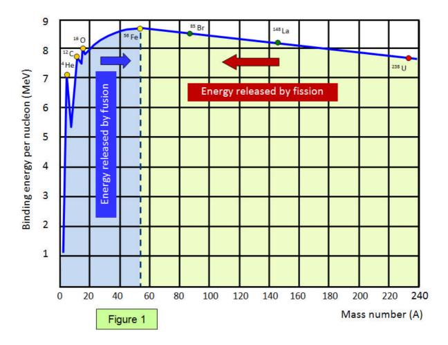
The part of the curve to the left shows that two light elements can produce energy by fusion while the part of the curve to the right shows that a heavy element can produce energy by fission. Notice that the diagram has been drawn with the binding energies per nucleon being shown as positive – this represents the energy needed to separate the particles.
